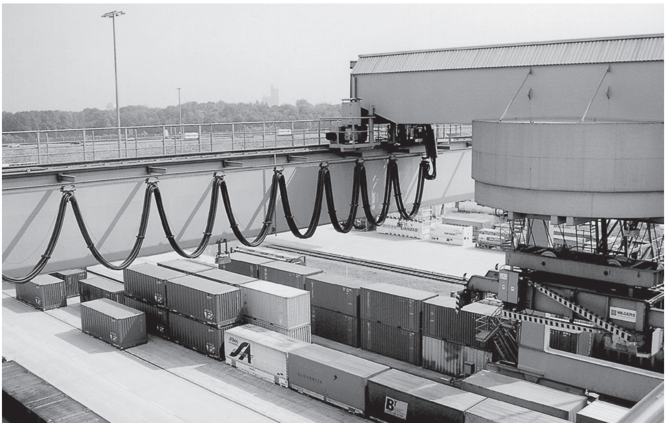
Cable carrier at a container crane
